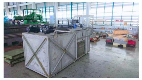
Full refurbishment of the grinding coolant system including new coolant filtration system.
