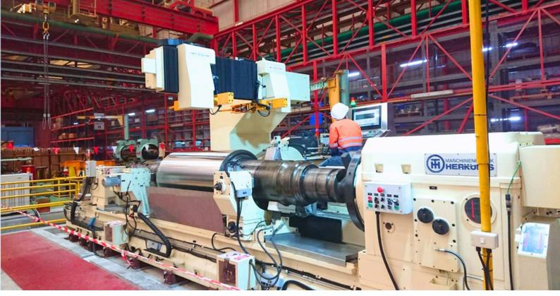
HERKULES WS450 AFTER RETROFIT GRINDING MIRROR FINISH ROLLS WITH WHEEL UP TO 500 GRIT.
