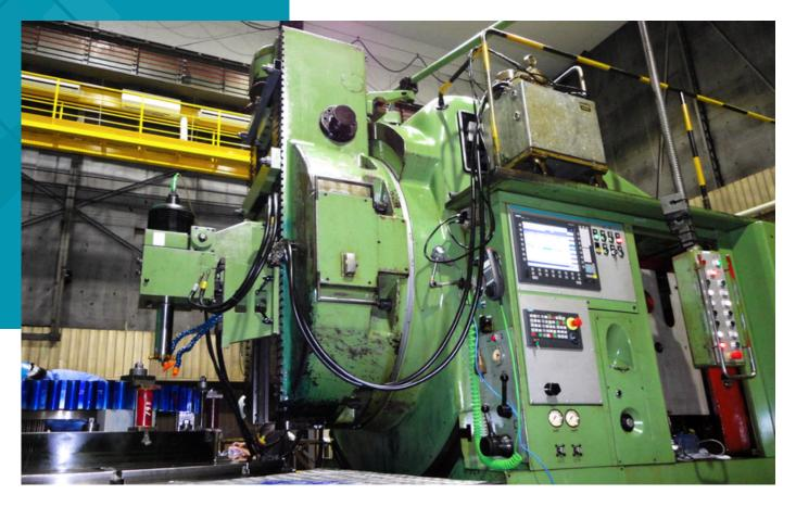
To align the MAAG SH600/735 with current technological standards while minimizing disruption, a strategic retrofit was proposed. The upgrade involved replacing the CNC NCU and operator panel components with the latest generation:
